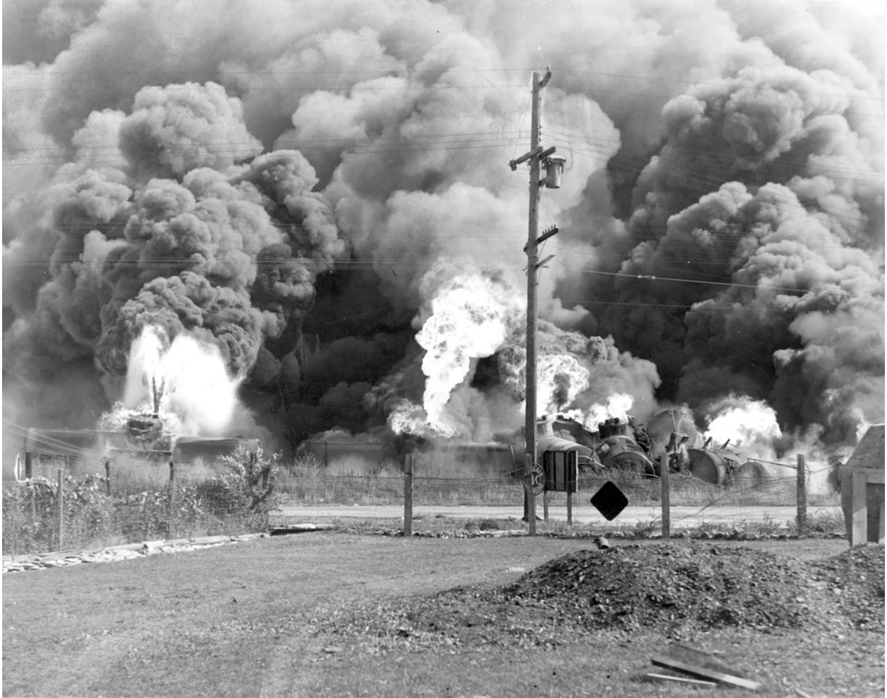
Ten tank cars burn as a Pennsylvania Railroad oil train is derailed by a dropped coupler. Nearly 100,000 gallons of oil went up in flame. Photo from Alex Campbell Collection.
